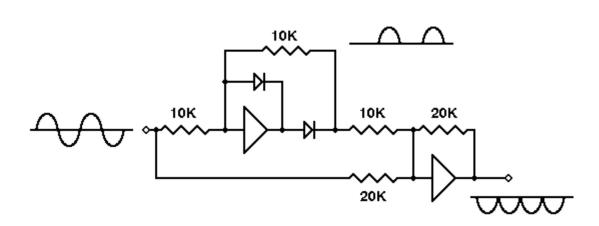
The circuit shown above performs full-wave rectification on the input signal, as shown. If you wish the final output to be positive instead of negative, simply reverse the two diodes in the half-wave rectifier section.
